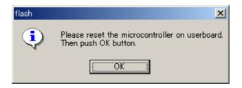
Downloading is performed to open the "Download" window. When downloading is completed normally, the following dialog window opens.
