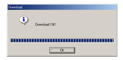
When the **[OK]** button is clicked to close the dialog window, the **[Erase]**, **[Blank Check]**, **[Program & Verify]**, **[Read & Compare]** and **[Copy]** buttons are enabled.
