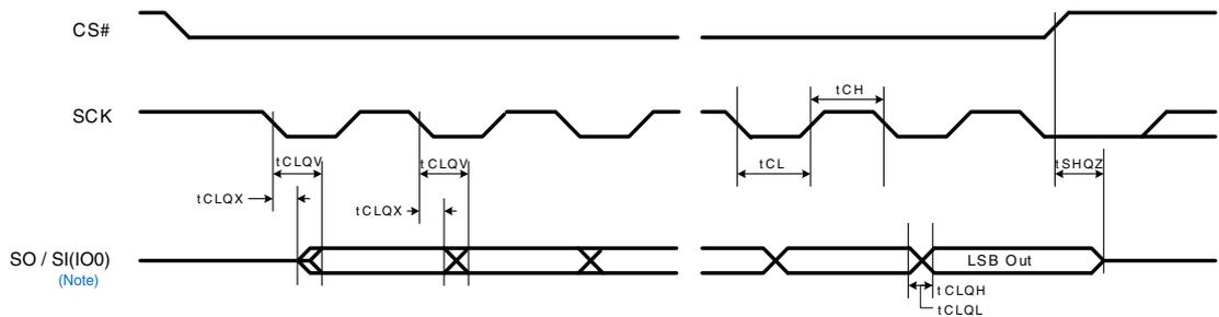
Note: SI(I/O) is an Output ONLY for the Fast Read Dual Output command (3Bh)
