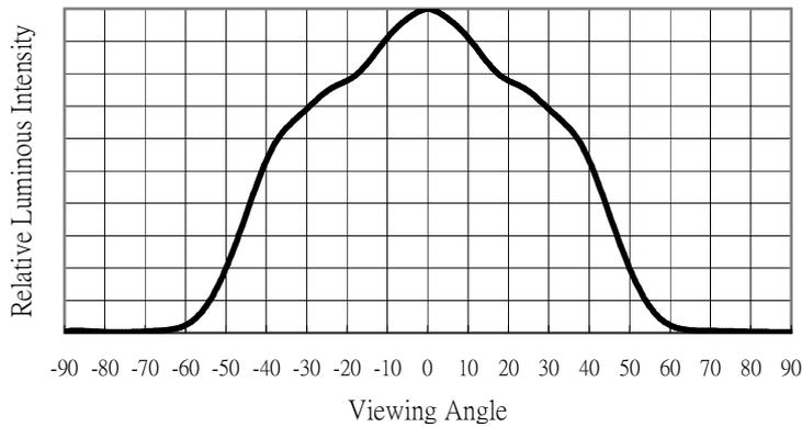
Fig. 5 Relative Luminous vs Viewing Angle
