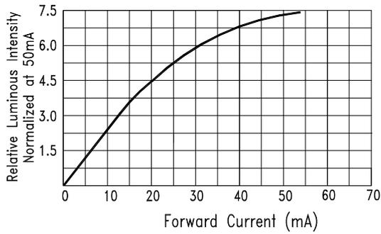
Fig.3 Relative Luminous Intensity vs. Forward Current
