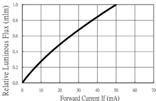
Fig.3 Relative Luminous Flux vs Forward Current
