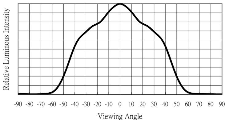
Fig. 5 Relative Luminous vs Viewing Angle
