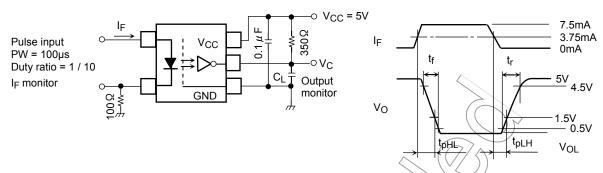
C<sub>L</sub> is approximately 15pF which includes probe and stray wiring capacitance.
