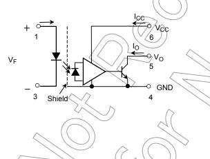
Note. A 0.1pF bypass capacitor must be connected between pins 4 and 6.
