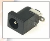
DC-10 PCB mounting pin / ring type with switch. Rated 12V / 5A. DC10A with 2.1mm dia. pin. DC10B with 2.5mm dia. pin. DC-10A (FC68148)
