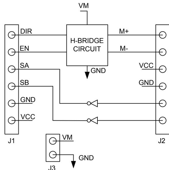
Motor power is provided via a two-pin terminal block (J3) that can accommodate up to 18-gauge wire. The HB5 circuits can handle motor voltages up to 12V.
