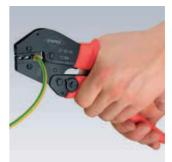
**Third step:** when greater hand force is required, such as e.g. when crimping insulated connectors 6 mm², two-hand operation is possible by the longer handles
