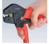
**First step:** move the handle with two fingers only until both jaws touch the connector to be crimped
