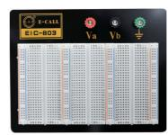
EIC-801D\*4PS EIC-801T\*3PS (1100 Tie-point) 3 Binding posts 5 Cushions
