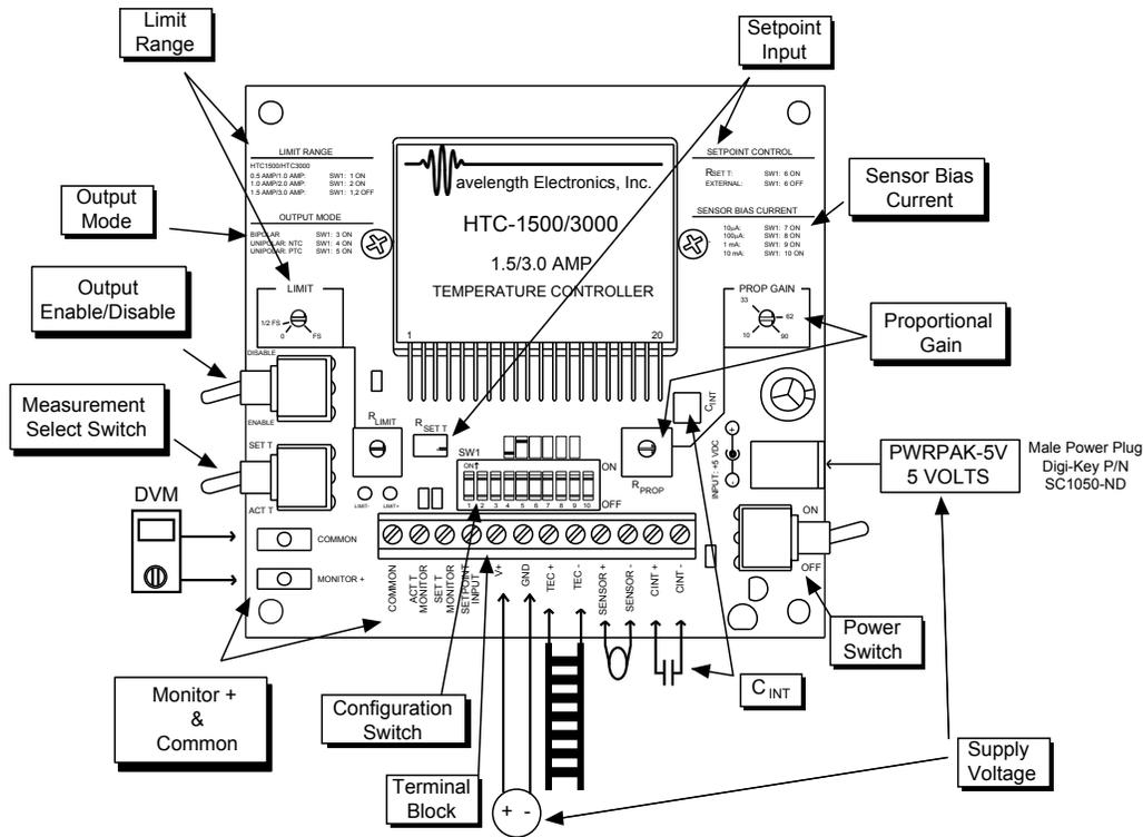
**To Install the HTC on the Evaluation Board with HTC Heatsink**
