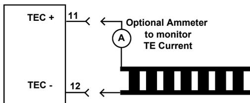
Connect the TE module and an ammeter if you want to monitor TE current. Current flows from positive to negative when the HTC is cooling with an NTC temperature sensor. When using an LM335, AD590, RTD, or other PTC sensor, reverse the polarity of the leads (i.e. connect the positive lead of the TE module to TEC- and the negative lead of the TE module to TEC+).
