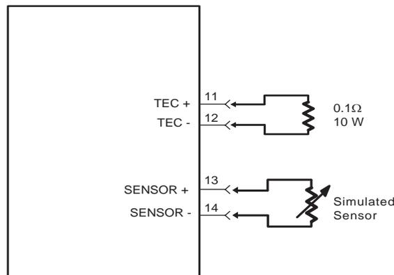
Values shown can simulate any load up to the HTC Series maximum of 3 A.
