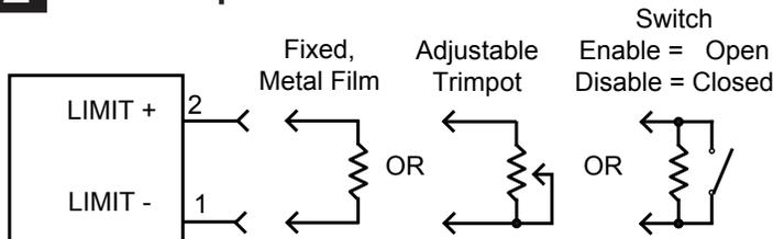
Use a trimpot no more than twice the calculated value of R<sub>LIMIT</sub> for best resolution.
