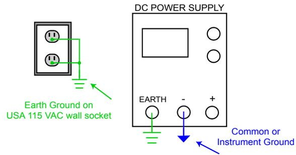
Unless Earth and Instrument Ground are connected via the power supply, Instrument Ground is floating with respect to Earth Ground
