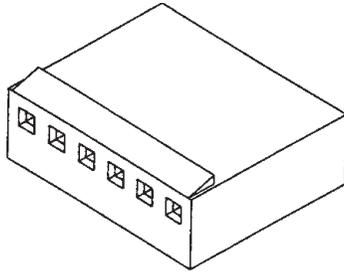
Molex Crimp Terminal Housing 20 pin (High Pressure)
