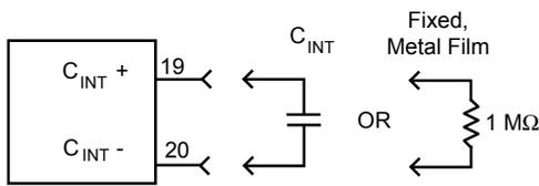
$$C_{INT} = \frac{T_{INT}}{1 \text{ M}\Omega}$$
