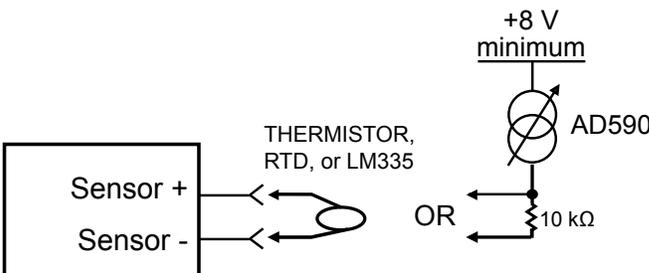
Virtually any type of temperature sensor can be used with the HTC. It must produce a feedback voltage between 0.25 V and (V+ minus 1.3 V). See Step #3 (R<sub>BIAS</sub>) to set the bias current to the sensor.
