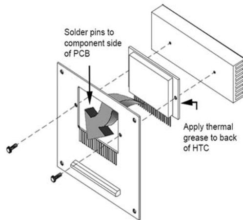
If the HTC is to be used without the evaluation PCB, apply the thermal grease as directed, line up the screw holes in the HTC and heatsink and attach with the supplied screws. Connect the HTC pins to your system by soldering them to the appropriate leads.
