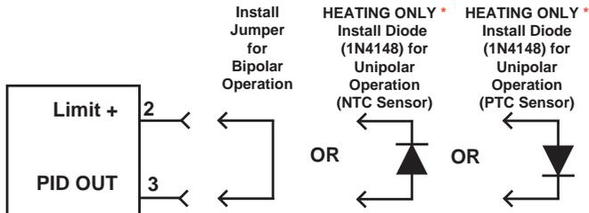
\* Do not install the diode if the HTCEVALPCB is used.
