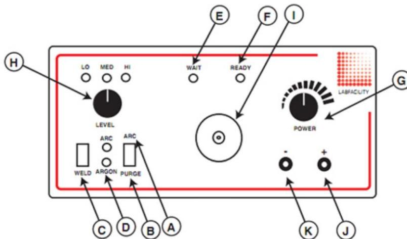
**A – ARC:** Argon gas and weld current controlled by the "Weld" switch. LED indication.
