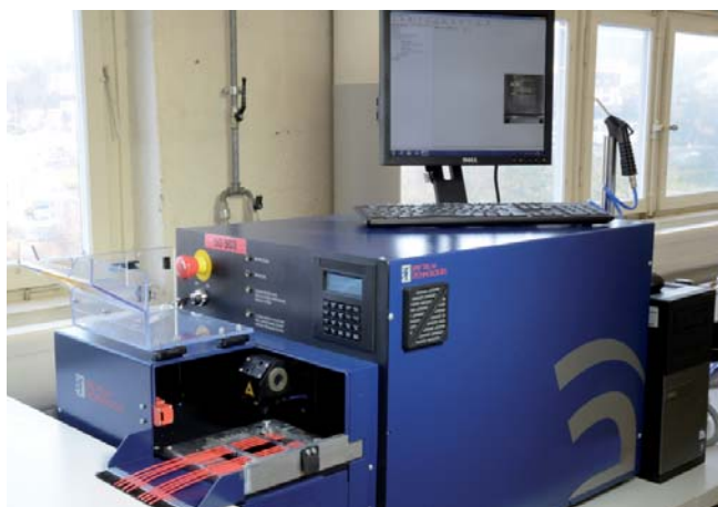
Automatic laser stripping
