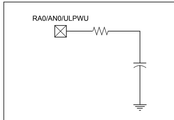
A timer can be used to measure the charge time and discharge time of the capacitor. The charge time can then be adjusted to provide the desired delay in Sleep. This technique compensates for the affects of temperature, voltage and component accuracy. The peripheral can also be configured as a simple Programmable Low-Voltage Detect (LVD) or temperature sensor.
