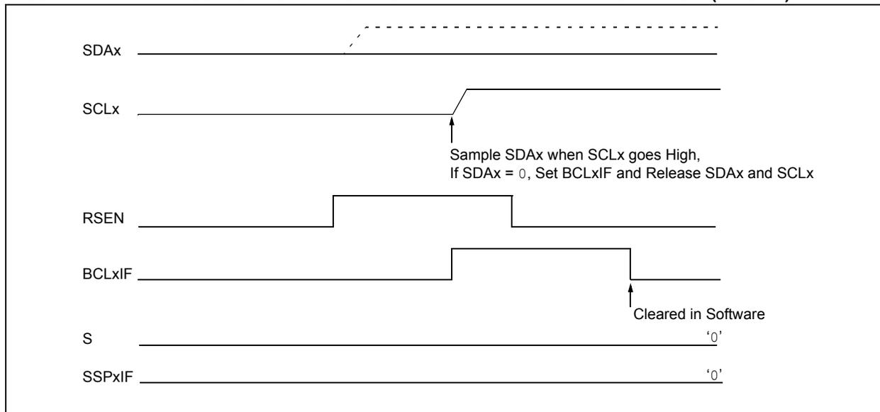
**FIGURE 21-32: BUS COLLISION DURING REPEATED START CONDITION (CASE 2)**
