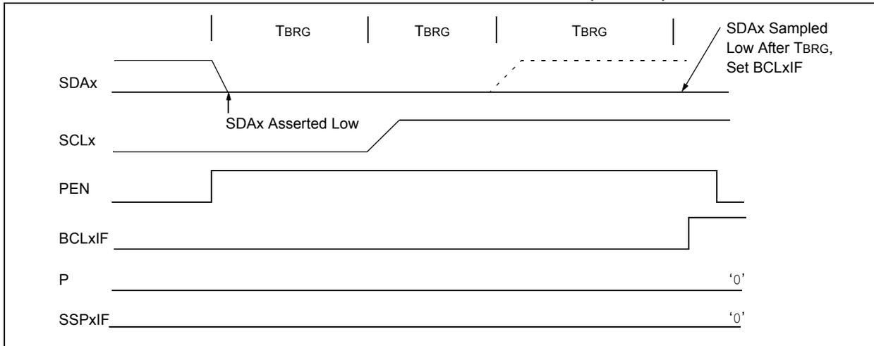
**FIGURE 21-34: BUS COLLISION DURING A STOP CONDITION (CASE 2)**
