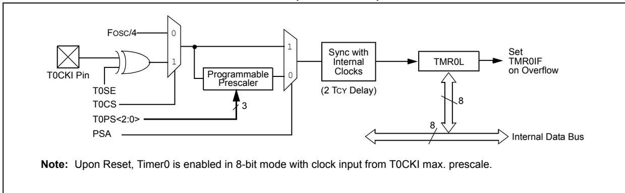
**FIGURE 13-2: TIMER0 BLOCK DIAGRAM (16-BIT MODE)**
