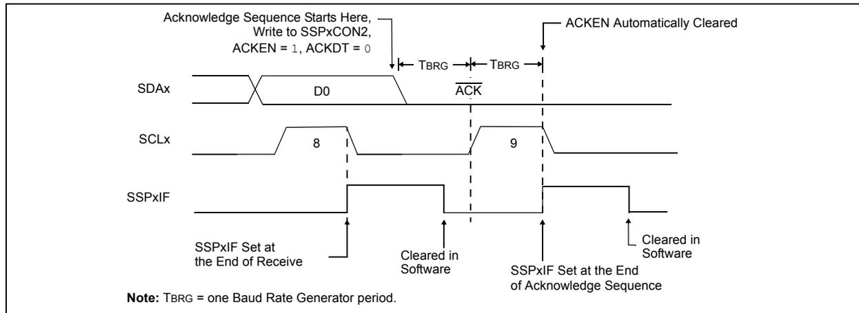
**FIGURE 21-26: STOP CONDITION RECEIVE OR TRANSMIT MODE**
