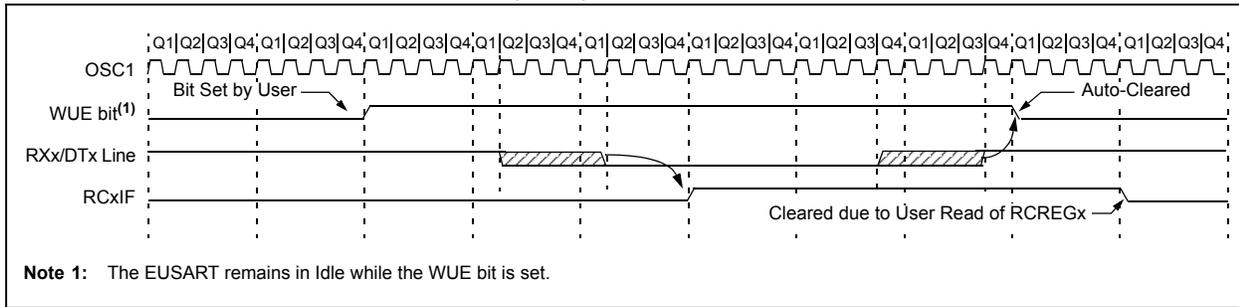
**FIGURE 22-9: AUTO-WAKE-UP BIT (WUE) TIMINGS DURING SLEEP**
