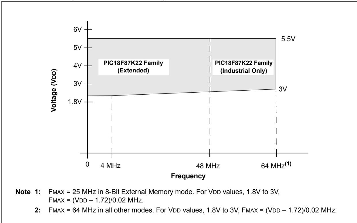
**FIGURE 31-2: VOLTAGE-FREQUENCY GRAPH, REGULATOR DISABLED (INDUSTRIAL/EXTENDED)<sup>(1,2)</sup>**
