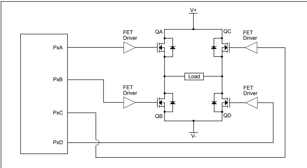
**FIGURE 20-9: EXAMPLE OF FULL-BRIDGE PWM OUTPUT**
