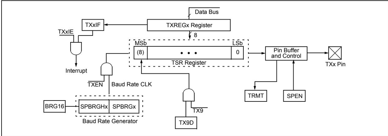
**FIGURE 22-4: ASYNCHRONOUS TRANSMISSION**
