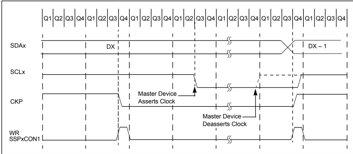
**FIGURE 21-15: I<sup>2</sup>C SLAVE MODE TIMING WITH SEN = 1 (RECEPTION, 7-BIT ADDRESS)**
