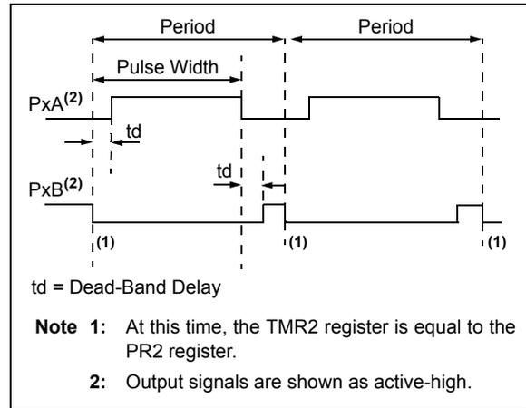
**FIGURE 20-7: EXAMPLE OF HALF-BRIDGE APPLICATIONS**
