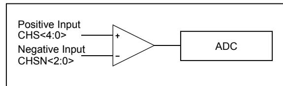
Differential conversion feeds the two input channels to a unity gain differential amplifier. The positive channel input is selected using the CHS bits (ADCON0<6:2>) and the negative channel input is selected using the CHSN bits (ADCON1<2:0>).
