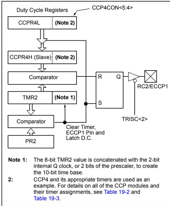
A PWM output (Figure 19-4) has a time base (period) and a time that the output stays high (duty cycle). The frequency of the PWM is the inverse of the period (1/period).
