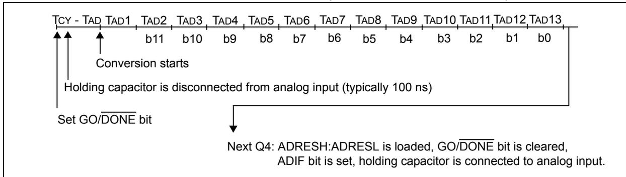
**FIGURE 23-7: A/D CONVERSION TAD CYCLES ( $\text{ACQT}\langle 2:0 \rangle = 010, \text{TACQ} = 4 \text{ TAD}$ )**
