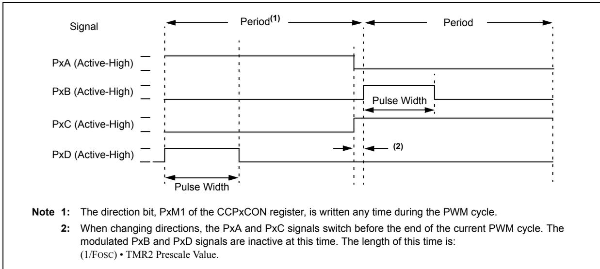
**FIGURE 20-11: EXAMPLE OF PWM DIRECTION CHANGE AT NEAR 100% DUTY CYCLE<sup>(1)</sup>**
