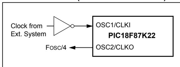
An external clock source may also be connected to the OSC1 pin in HS mode, as shown in [Figure 3-6](#). In this configuration, the divide-by-4 output on OSC2 is not available. Current consumption in this configuration will be somewhat higher than EC mode, as the internal oscillator's feedback circuitry will be enabled (in EC mode, the feedback circuit is disabled).
