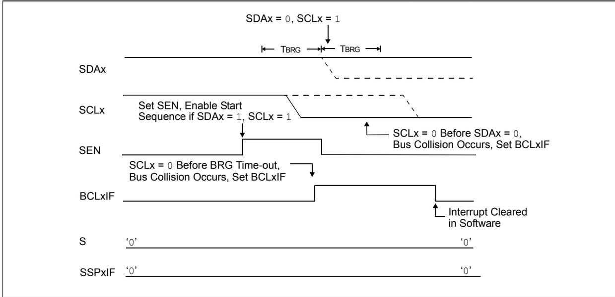
**FIGURE 21-30: BRG RESET DUE TO SDAx ARBITRATION DURING START CONDITION**
