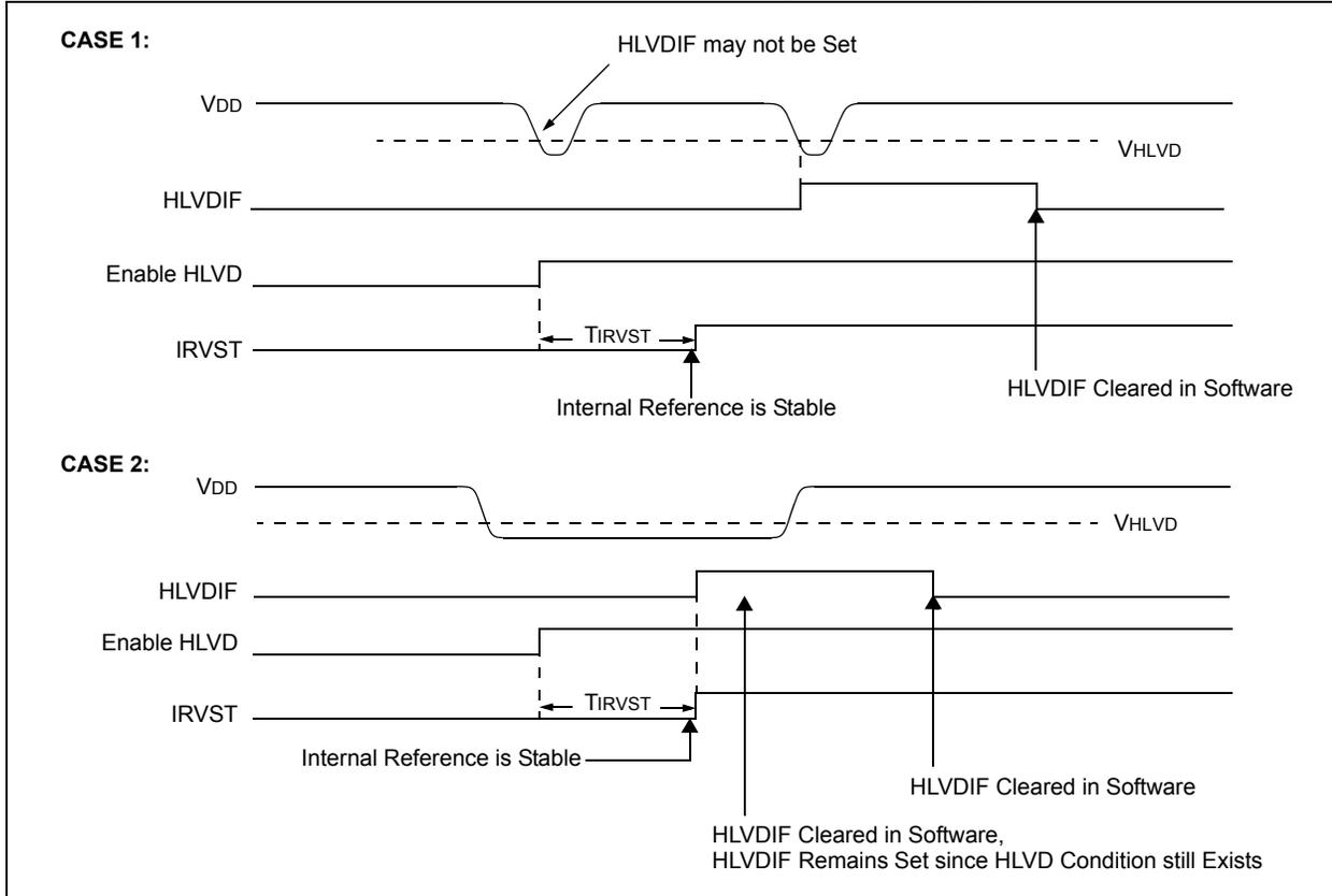
**FIGURE 26-3: HIGH-VOLTAGE DETECT OPERATION (VDIRMAG = 1)**
