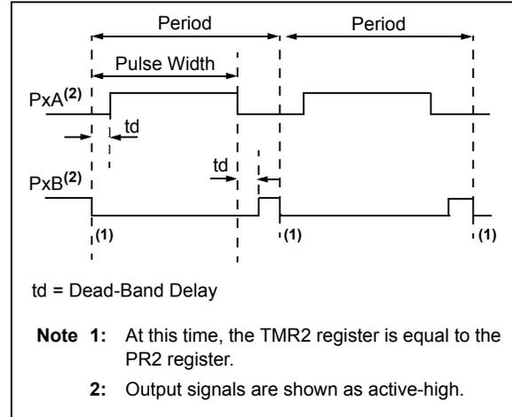
**FIGURE 20-15: EXAMPLE OF HALF-BRIDGE APPLICATIONS**
