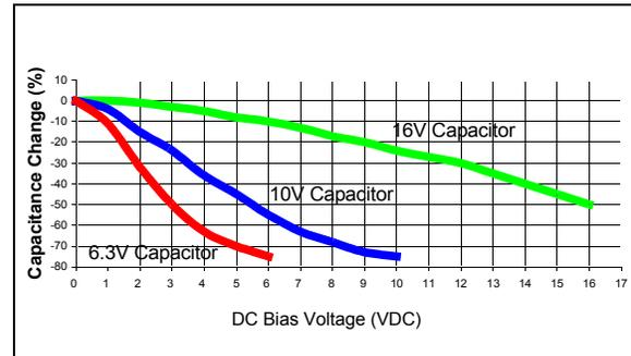
When selecting a ceramic capacitor to be used with the internal voltage regulator, it is suggested to select a high-voltage rating, so that the operating voltage is a small percentage of the maximum rated capacitor voltage. For example, choose a ceramic capacitor rated at 16V for the 2.5V core voltage. Suggested capacitors are shown in [Table 2-1](#).
