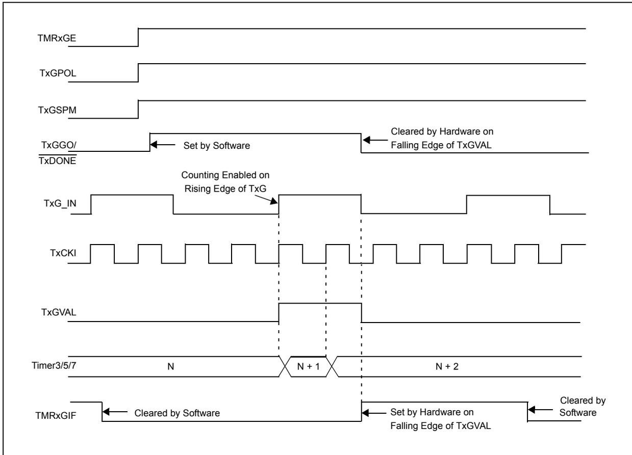
**FIGURE 16-5: TIMER3/5/7 GATE SINGLE PULSE AND TOGGLE COMBINED MODE**
