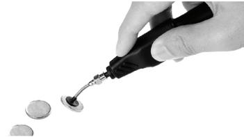
→ For best performance, the object should have a flat, clean, dry, non-porous surface, and be within the rated load. See "Technical Data" for suction cup (1) size / load.
