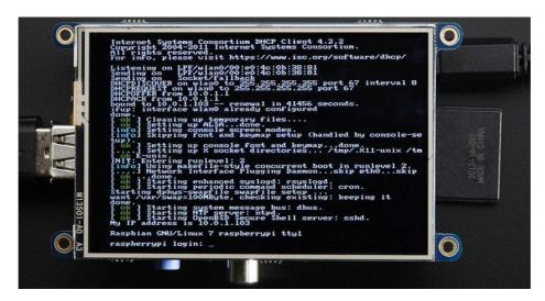
It's designed to fit nicely onto the Pi Model A or B but also works perfectly fine with the Model B+ as long as you don't mind the PCB overhangs the USB ports by 5mm.
