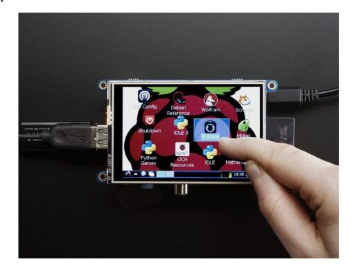
Is this not the cutest, little display for the Raspberry Pi? It features a **3.5"** display with **480x320** 16-bit color pixels and a resistive touch overlay, but is only slightly larger than our popular original (https://adafru.it/dDE). The plate uses the high speed SPI interface on the Pi and can use the mini display as a console, X window port, displaying images or video etc. Best of all it plugs right in on top!
