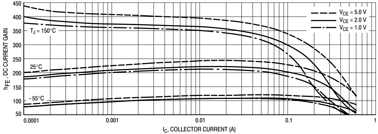
Figure 12. DC Current Gain
