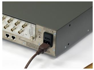
Connect the plug of the power cord to a grounded AC outlet.
