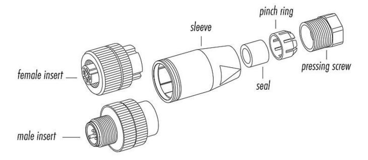
material of locking rings: plastic, zinc diecast, stainless steel
