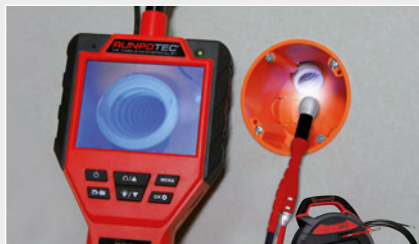
Pipe inspection from Ø 14 mm and more
