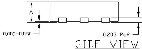
NOTE: The exposed solder pad (on the bottom of the package) is not electrically connected to any other pin (isolated).
