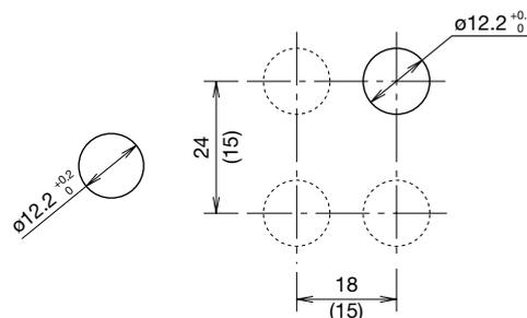
Note: (15) is the minimum mounting hole layout without AC adapter or flasher unit.
