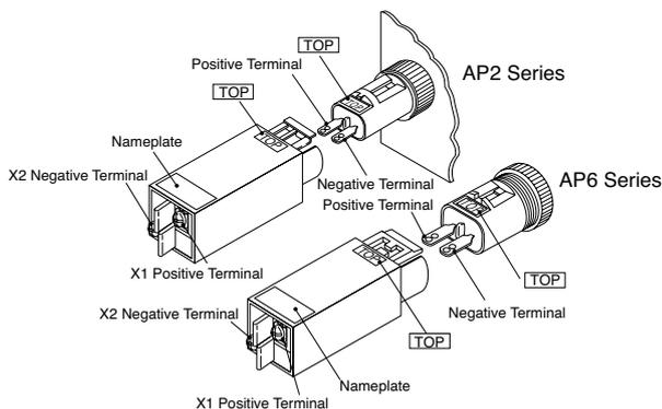
Note: Do not apply excessive force to terminals X1 and X2 during wiring.
