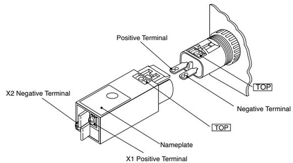
Note: Do not apply excessive force to terminals X1 and X2 during wiring.
