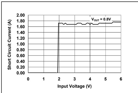
**FIGURE 2-21:** Short Circuit Current vs. Input Voltage.
