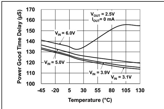
**FIGURE 2-9:** Power Good (PWRGD) Time Delay vs. Temperature.
