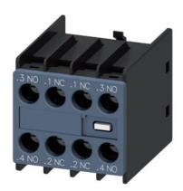
auxiliary switch, on the front, 2 NO + 2 NC, .3/.4, .1/.2, .1/.2, .3/.4, current path: 1 NO, 1 NC, 1 NO, screw terminal, for contactors 3RT2 and contactor relays 3RH2
