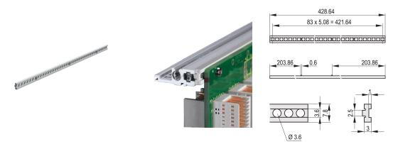
Strip enables an insulated mounting of backplanes or metal plates as supports for connectors. Creates standardized mounting depth for plug-in units in the subrack in conjunction with L-ST and H-ST horizontal rails. Suitable for RatiopacPRO/-AIR, Propac Pro, CompacPRO and EuropacPRO/-Rugged.
