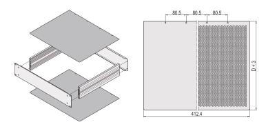
Cover plates plain will close the 19" chassis on top and bottom side. They protect the chassis from parts that could fall into the chassis.
