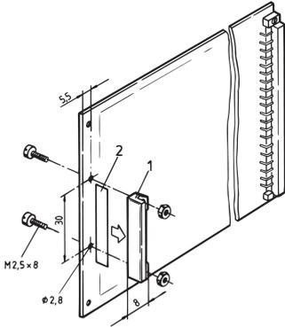
The PCB handle enables a user to extract a PCB without a front panel.
