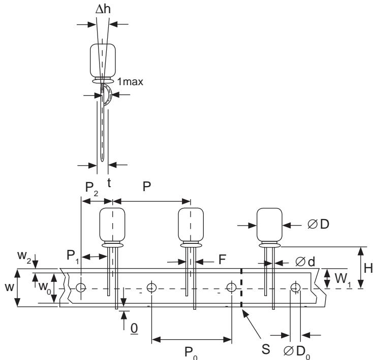
**NOTE:** ANODE (+) LEAD FEEDS OFF FIRST.
