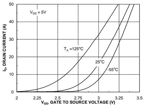
Figure 5. Transfer Characteristics.
